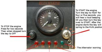
The Battery warning lights The Engine temperature Warning The Low Oil warning light
