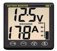
The battery power indicator above is the display for the 'Domestic' battery bank. It shows how charged the batteries are which power the lights, fridge, tv and radio when the engine is not running. The little bars displayed on the right hand side show the amount of power there is. Here it is showing that the batteries have about 60% power left: When the indicator gets down to about 30-40% you should start the engine and run it for an hour or so to re-charge the batteries.
